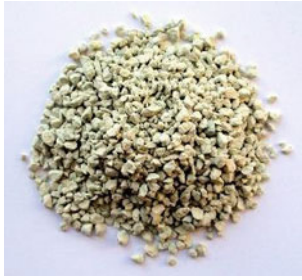
Fig. 2.5 Natural zeolite (clinoptilolite) granulated mineral
